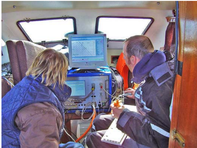
Fig. 3 Parametric echosounder acquisition unit (below) and navigation laptop (top) on board a small survey vessel. (© RCMG Universiteit Gent).
