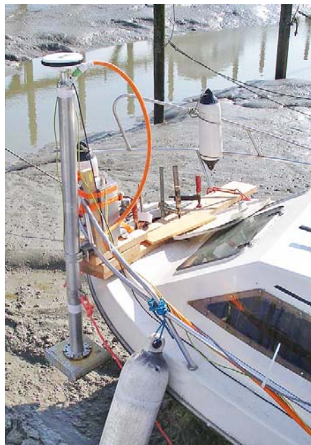
Fig. 2 Parametric echosounder transducer mounted onto a pole attached to the front of a small vessel. A GPS antenna is attached to top of the pole. Next to the pole a motion sensor is mounted on the deck. (© RCMG Universiteit Gent).
