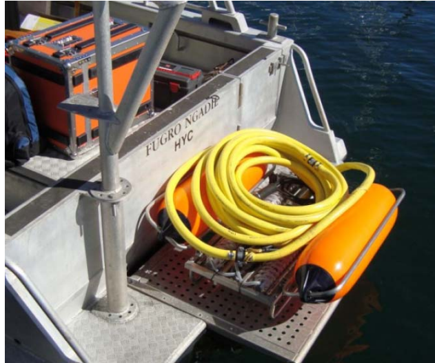
Fig. 1 Multi-tip sparker, cable and floaters (© Geo Resources)
