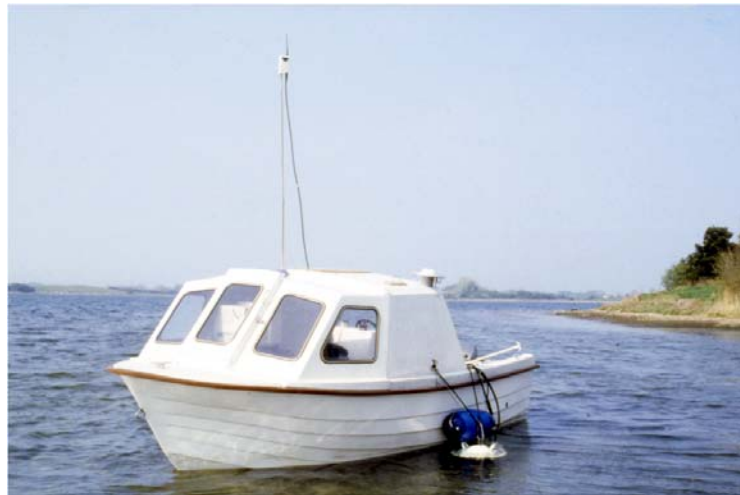
Fig. 2 Small boat with chirp towfish deployed on the side; the fender protects it against vibrations from the hull. © Ole Grøn.
