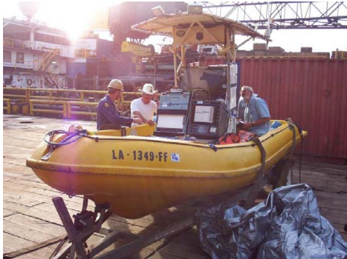
Fig. 3 Typical small boat used for echosounder survey.
