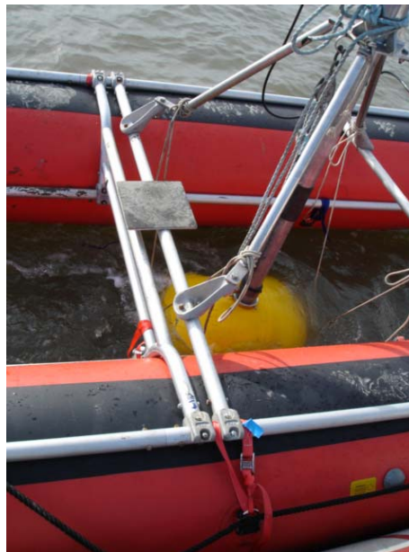
Fig. 2 Echosounder towfish mounted on a floatable platform.
