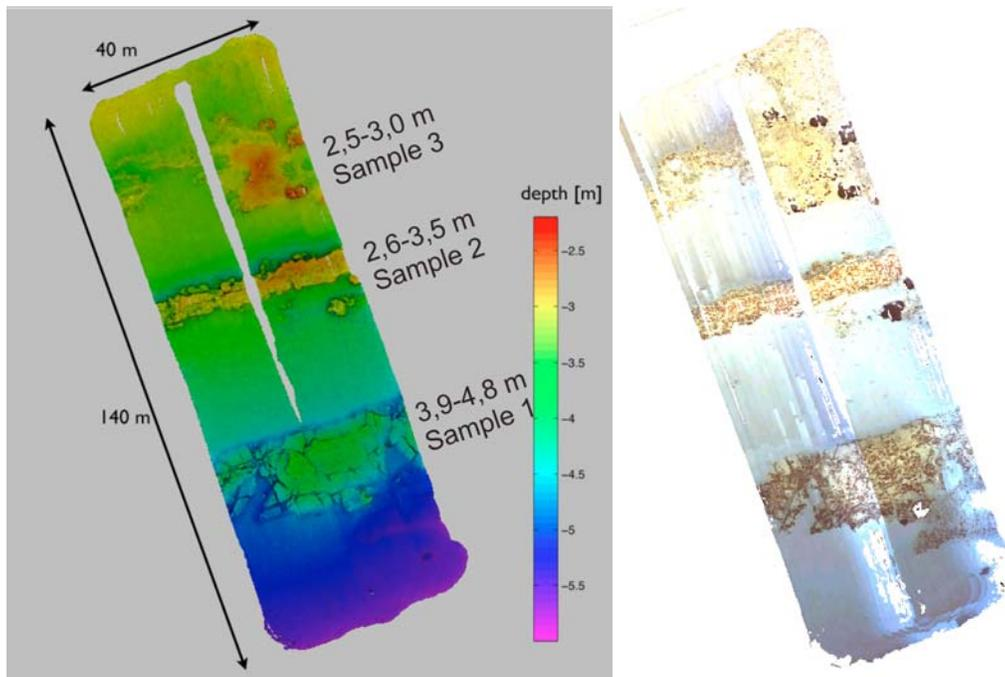
Figure 8: Two views of the 3D reconstruction from AUV-conducted optical imagery, Vatika Bay, SE Peloponnese, Greece. 3D structure shaded by depth (left) and with the optical images projected back onto the 3D surface (right) to form a 3D mosaic. The three bands of beach-rock are clearly visible. Core samples depths are indicated (above left) (Pizarro et al, 2012).
