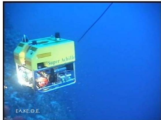
Fig. 4: Super Achilles ROV, 600m (HCMR)
