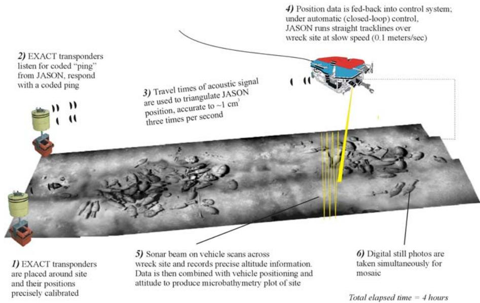
Fig. 7: Jason ROV conducting photographic survey ("closed loop control") above Wreck D in Skerki Bank in 1997 (drawing by D. Mindel from Oleson & Adams, 2004)
